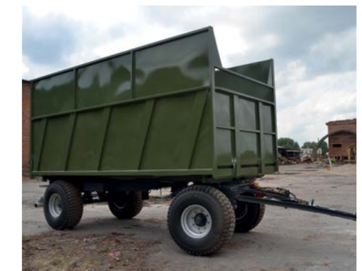
2TSP-14 chip carriers with a body volume of 24 m 3
