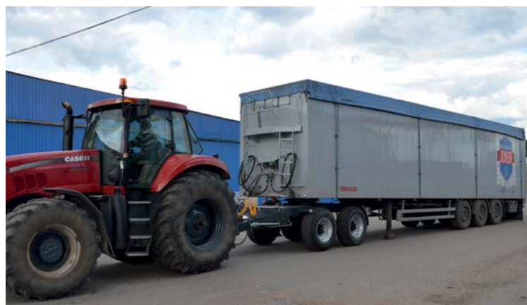
Connection of PSP-20 Dolly with a truck semi-trailer and tractor
