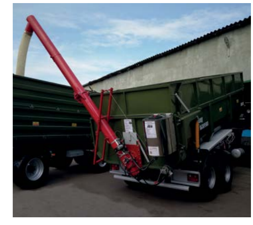
Auger on trailer with rear unloading
