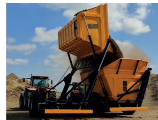
The maximum unloading height is 4,000 mm
