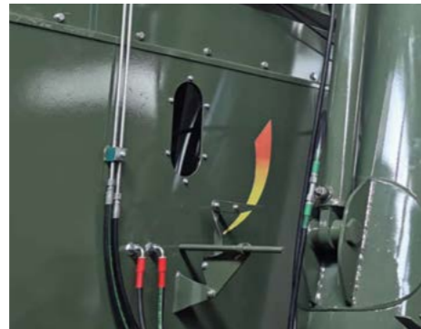
Indicator of slide gate opening
