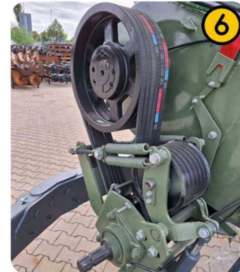
Separate drive with alternate inclusion of augers. The drive of the vertical auger is directly through the gearbox, of the horizontal auger - through the belt transmission
