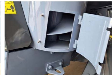
One hatch for cleaning of vertical auger
