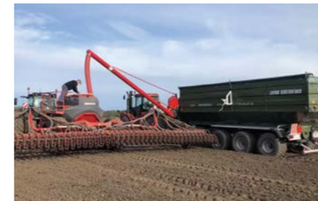
Loading of seeding machines through PVC hose
