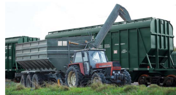
Extended auger h-5.5 m for loading wagons
