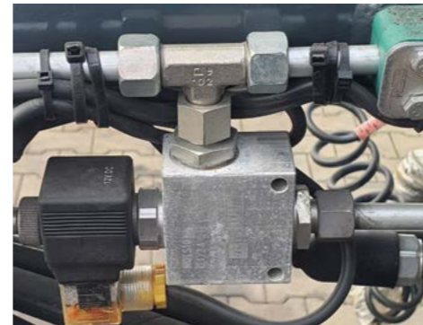
Hydraulic valve to block opening of the sliding gate at fixed PTO
