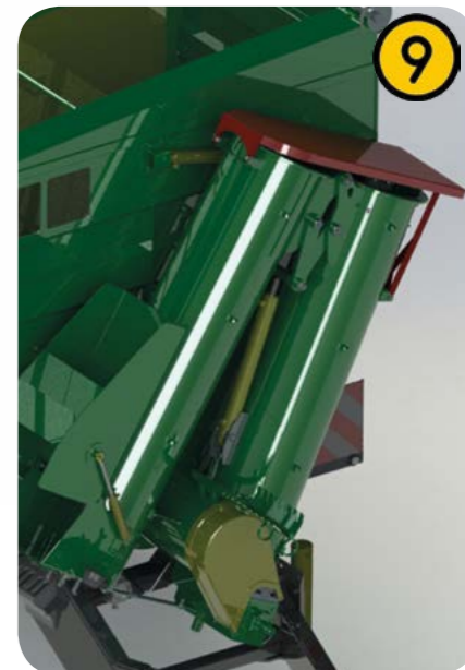
Protective cover of the auger against precipitation
