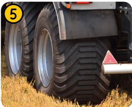
Maximum wheel size 850/40R26.5 - Minimum ground pressure 1.5 kg/cm 2
