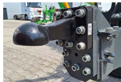
Adapter for height adjustment to hitch to any tractor
