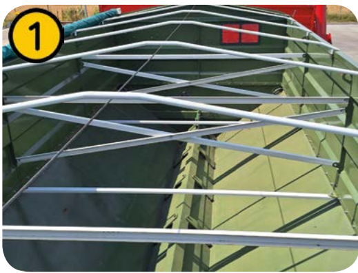
The sides of the body are pulled together by powerful profile spacers
