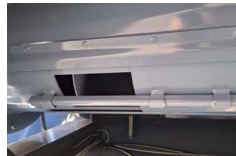
Three cleaning flaps of horizontal auger
