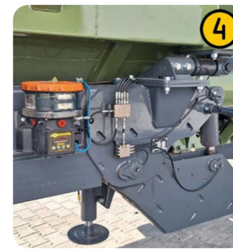
Programmable computer with precise bearing lubrication interval
