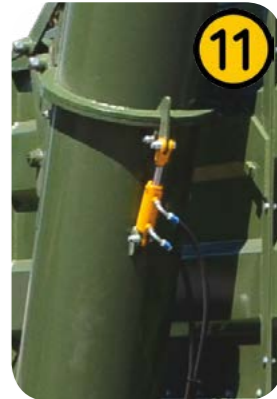
Hydraulic lock of two auger parts
