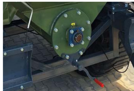
Screw mechanism of opening of horizontal auger cleaning flap
